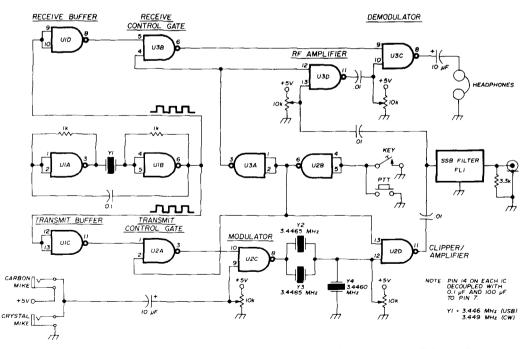
fig. 5. Schematic diagram of a complete ssb transceiver using 7400 series ICs. Circuit for ssb filter, FL1, is shown in fig. 6.
